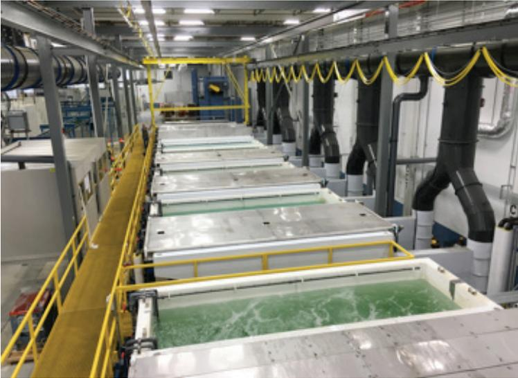
Figure 3: Automatic line and smart tank covers integrated into the exhaust system.
