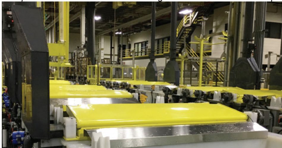
Example of automatic tank covers integrated with ventilation dampers
