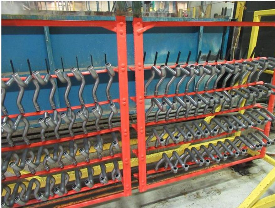
**Figure H-10. Racks with New Plastisol Coatings**
