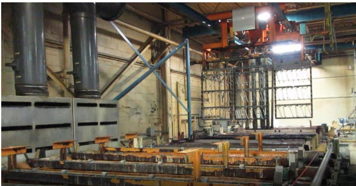
Figure H-1. Automated Zinc/Nickel Rack Plating Line
