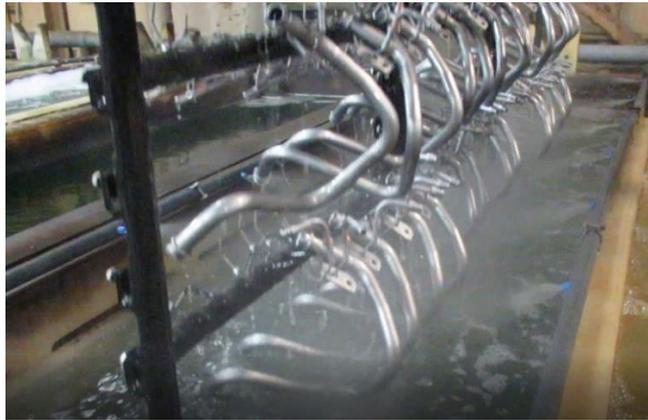
*Figure H-6. Spray Rinse on Tank 111*
