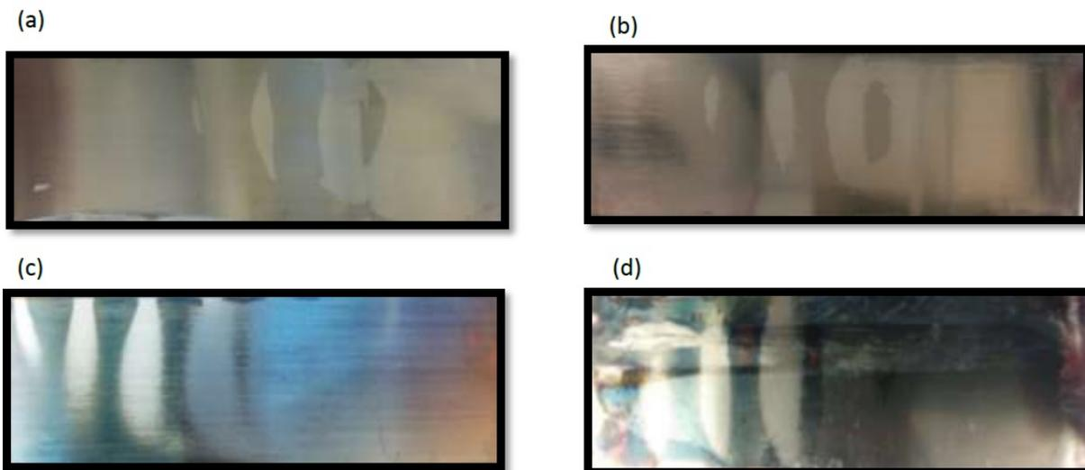
Figure 9 - Ni-W deposit along a Hull cell with (a) no BD, (b) 1 mM BD, (c) 2.5 mM BD and (c) 5 mM BD, at pH 8.
