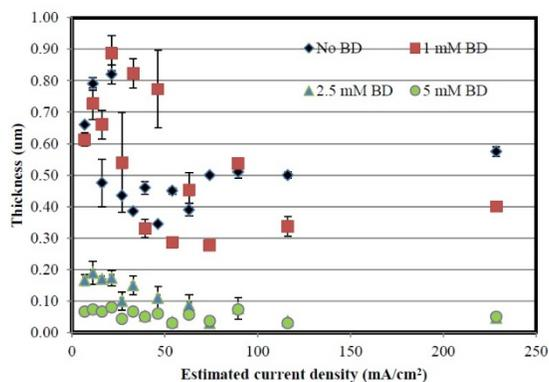
Figure 8 - Deposit thickness of Ni-W deposits at pH 8.
