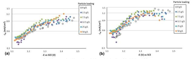
Figure 4 - Partial current densities with variable particle loading: (a) nickel and (b) tungsten.
