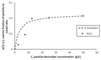
Figure 3 - Volume fraction ratio,  $\alpha/(1 - \alpha)$ , as a function of the particle electrolyte concentration comparing data with Gugliemi's model with fitted constants, cathodic current density = 28 mA/cm² (-1.2 V<sub>SCE</sub>).
