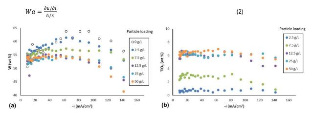
Figure 2 - Ni-W-TiO<sub>2</sub> deposit composition with variable particle loading: (a) wt% tungsten and (b) wt% TiO<sub>2</sub>.
