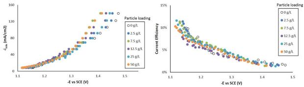
Figure 5 - Side reaction with variable particle loading.
