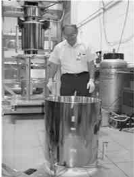
Figure 15 - Ni-Co-P alloy large x-ray mirror test cylinder (Photo courtesy of University of Alabama, Huntsville, AL).
