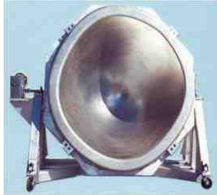
Figure 11 - Stationary and pivoting lay-up tools for composite aircraft radomes (Left photo courtesy of Bone Engineering Corp., Glendale, CA; right photo courtesy of Nickel Institute).
