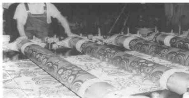
Figure 5 - Printing with electroformed nickel screen cylinders (Photo courtesy of Nickelmesh AG, Rudolfstetten, Switzerland).
