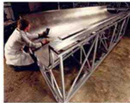
Figure 12 - Electroformed lay-up tools for aircraft wing fairings (Left photo courtesy of Galvanoform GmbH, Lahr, Germany; Right photo courtesy of Airbus/Nickel Institute).
