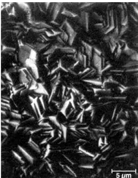
Figure 6 - Surface morphology of a commercial electrogalvanized coating (SEM: 3000×).
