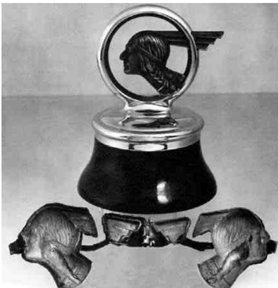
Figure 1 - Radiator cap/hood ornament for a 1930s Pontiac showing the original copper electroform configuration.
