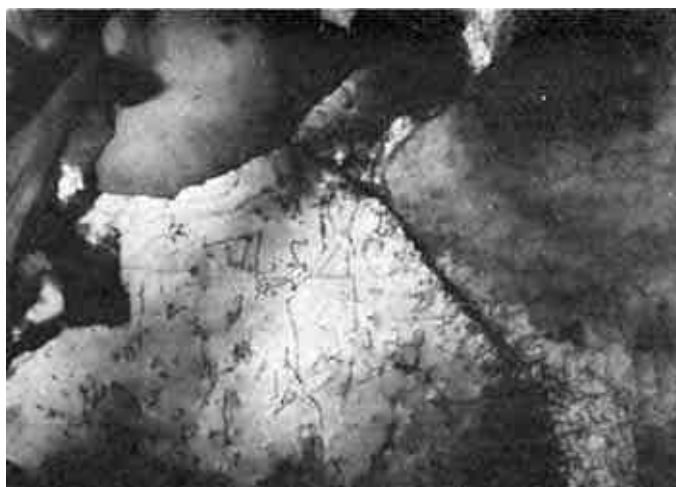
Figure 20 - Electron transmission micrograph of thinned, as-plated nickel deposit from Watts bath. Original magnification: 40,000 \times .
