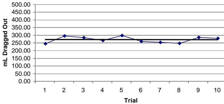
Figure A-10 - Graphed Raw Dragout Data - Barrel Design 4 - Trial 1
