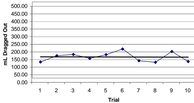
Figure A-13 - Graphed Raw Dragout Data - Barrel Design 5 - Trial 1
