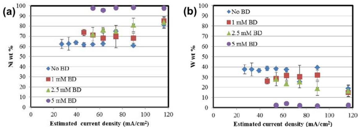
Figure 4 - Alloy composition as a function of current density: (a) nickel and (b) tungsten.
