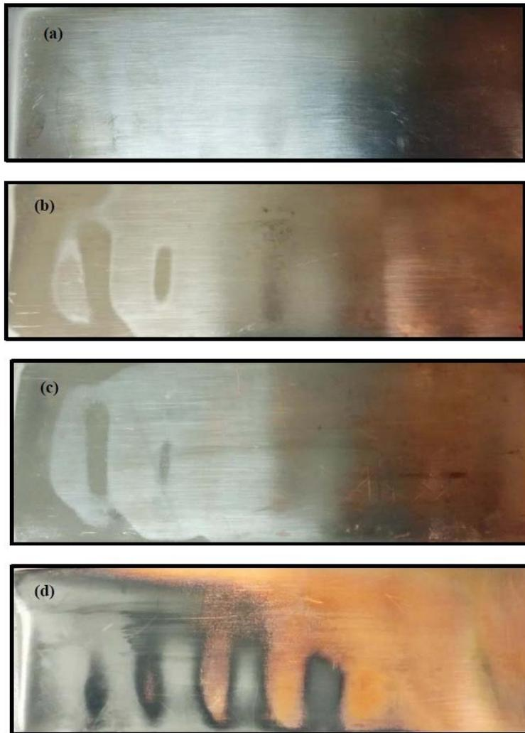
Figure 2 - Photographs of Ni-W deposit with varying amounts of BD at an average current density of  $-50 \text{ mA/cm}^2$ : (a) No BD, (b) 1 mM BD, (c) 2.5 mM BD and (d) 5 mM BD.
