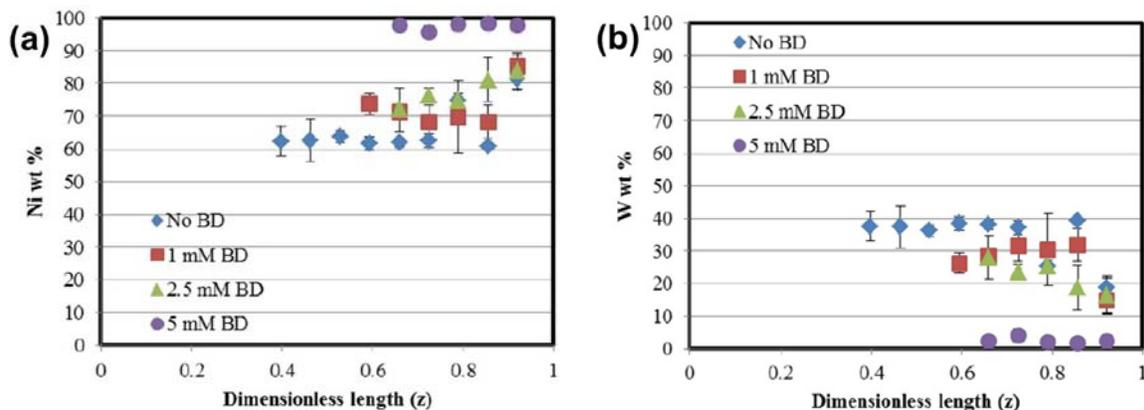
Figure 3 - Alloy composition as a function of cathode length: (a) nickel and (b) tungsten.
